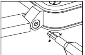
The 4 socket head screws (hexagon socket/1.3 mm diameter) mount the strap to the case attachments. These screws must be handled carefully, using the 2 tools supplied with the watch in its box.
