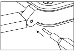
A spring bar is used to fit the strap to the case attachments. This bar must be removed carefully using the appropriate tool provided with the watch in the box.
