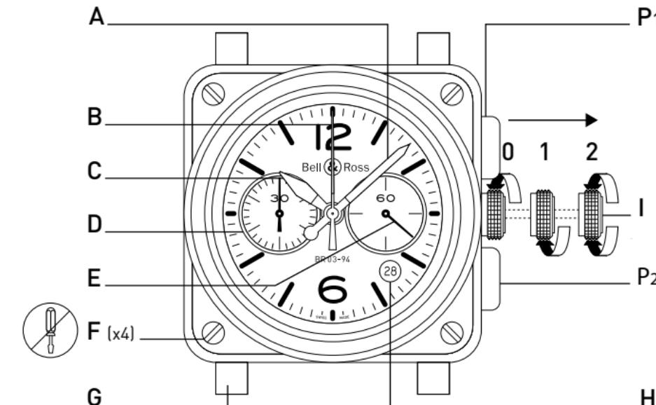
0. Wind the movement manually (rotate clockwise)
